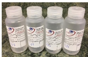
250 mL plastic containers for PFAS sampling.
